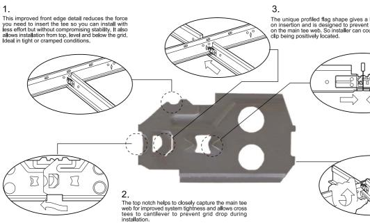
The unique profiled flag shape gives a loud click on insertion and is designed to prevent snagging on the main tee web. So installer can count on the
